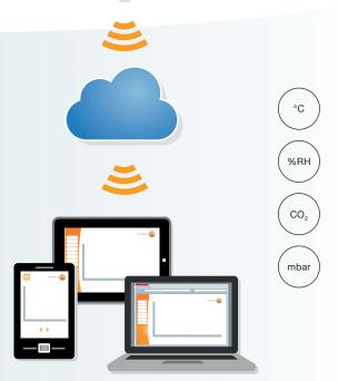
The WiFi data logger testo 160 IAQ monitors the ambient conditions temperature, humidity, atmospheric pressure and the CO<sub>2</sub> concentration in buildings such as public facilities, office complexes and education institutions. The logger transfers measurement values by wireless LAN to the online store (Testo Cloud). You can access all data at any time via your normal browser on your PC/tablet/ smartphone. If limit values are exceeded, an alarm is immediately provided by SMS and/or e-mail.
